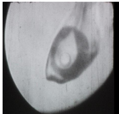
Fig 1: "This CO 2 bubble is growing or disappearing: (phase equilibrium vs. temperature)". This movie was the sensation of the International Geological Congress of 1952 and the trigger for the later interest for fluid inclusions
