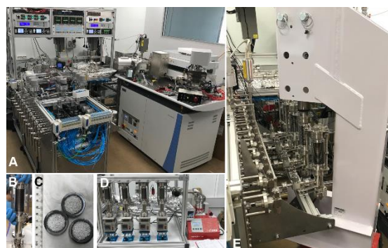
Fig. 1: Experimental set up: A - Automated NG machine at CSIRO, B - Assembly of one crusher container, C - WC sample plates filled with 1mm quartz grains, D - Pre-vacuum system for crusher container, E -Crusher container connected to NG line including press
